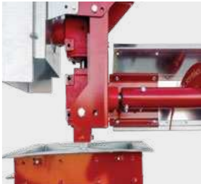
Double gearbox to get the sweep lower to the bin floor
